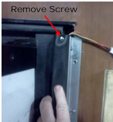
Figure 4 Removing the bulb seal screw
